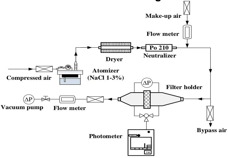
$$\eta(\%) = \left(1 - \frac{C_{downstream}}{C_{upstream}}\right) \times 100\%$$
