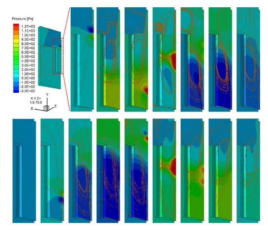
Evolution of static pressure contours and flow streamlines when the opposing puled-jet cleaning was operated with the delay time of 0.075 s (a) and -0.075s (b) while keeping PR=1.0
